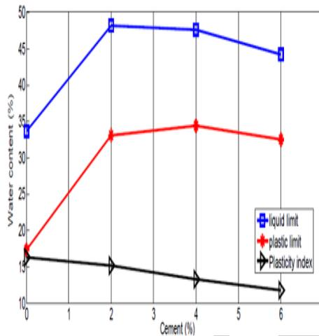
Fig.5.2 shows the effect of addition of cement on Atterberg's limits. It is observed that there is an increase in both liquid limit and plastic limit at 2 percent cement and thereafter both limits remain fairly constant. Plasticity index have very small change with increasing the percentage of cement. The initial increase in liquid limit indicates flocculation of soil particles due to addition of cement.
